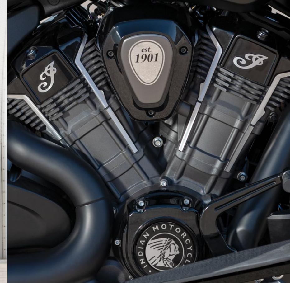
Our all-new liquid-cooled PowerPlus V-twin is the most powerful engine in its class. With overhead camshafts and four valves per cylinder delivering a blistering 122hp and 128 ft-lbs of torque, it redefines ultimate bagger performance.
